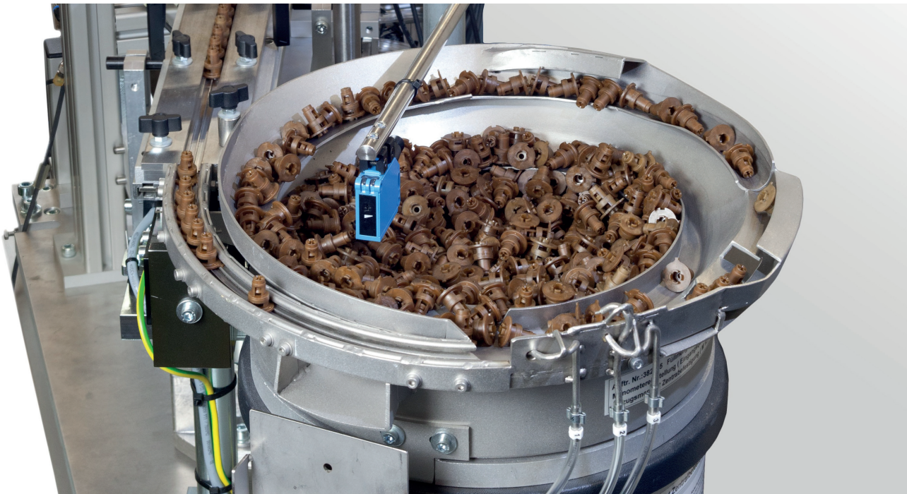
Typical application: SRC-N 250-2 with ZSB-Z 250 for feeding of cases
